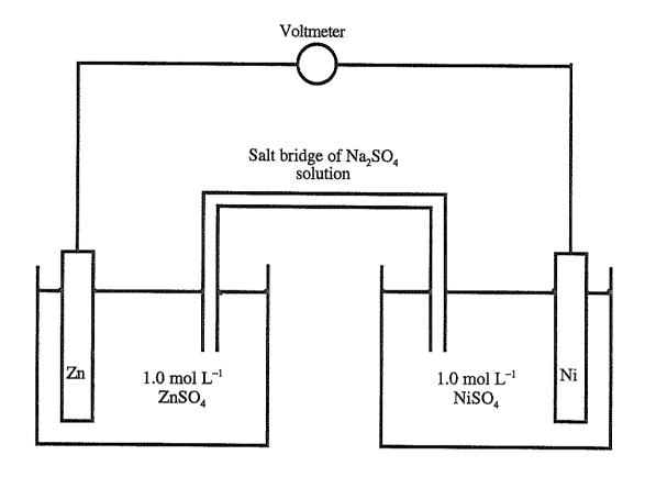
(a) Write the half-equation for the reaction occurring at the cathode.
